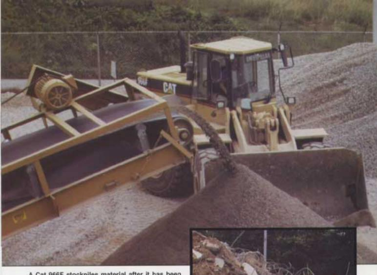
A Cat 966F stockpiles material after it has been processed in the crushers. A number of recycled construction materials – including #57 stone for use as drain fill, crusher run for use as base, and #67 aand #810 screenings for paving aggregate applications – are being produced at the site. Much of it will be used in new development at the site. At right: Typical material before processing.
